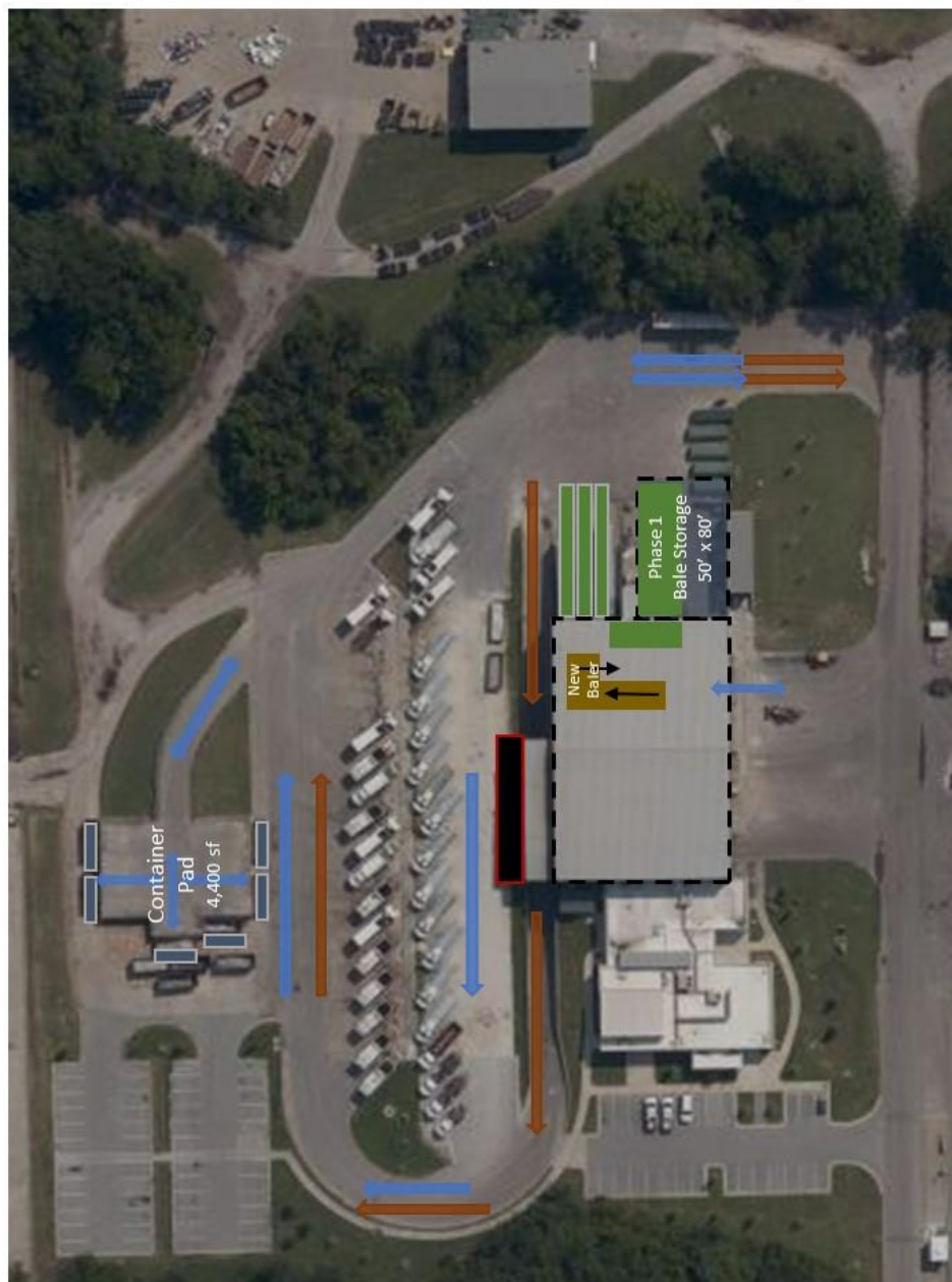
Figure 6: Fayetteville, AR RPF Conceptual Site Plan – Option 3 (Expanded Bale Storage)
