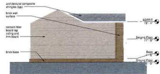
4 West Elevation 1/8" = 1'-0"
