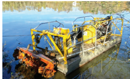
Dino 6 dredge owned and utilized by Stream Lake and Wetland Solutions LLC to remove sediment from the lake.
