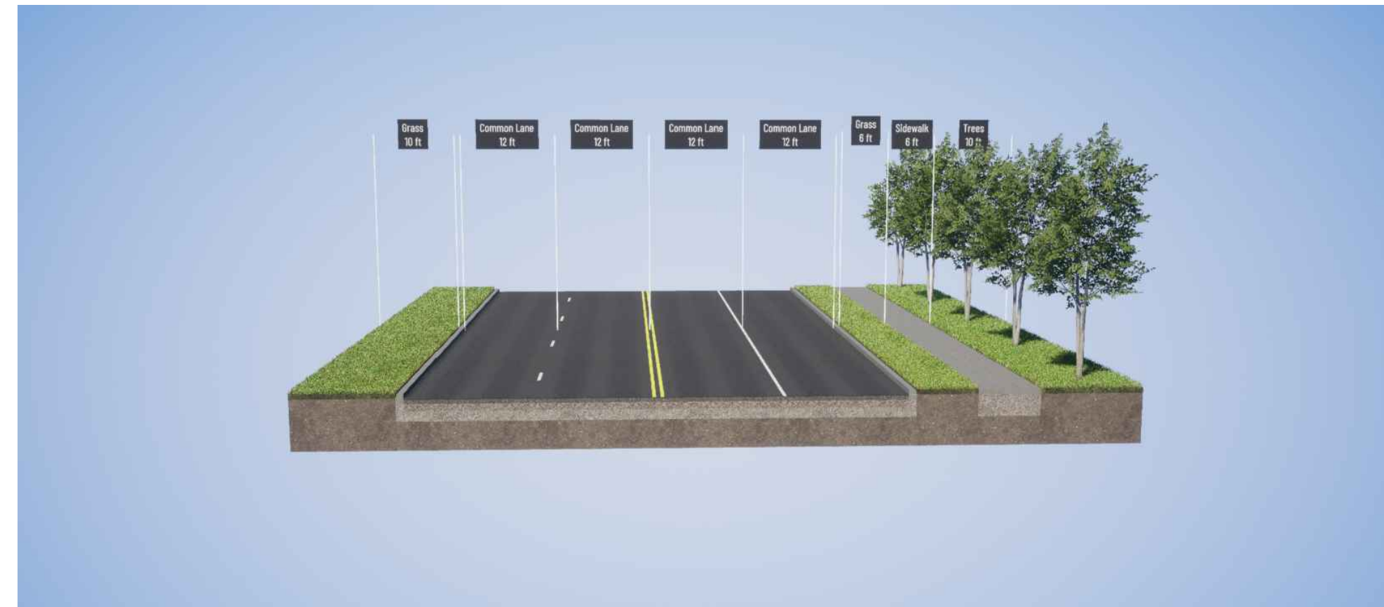
EXISTING TYPICAL SECTION
