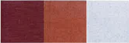
rainscreen panel system options: composite metal, terracotta panel, cement fiberboard panel
