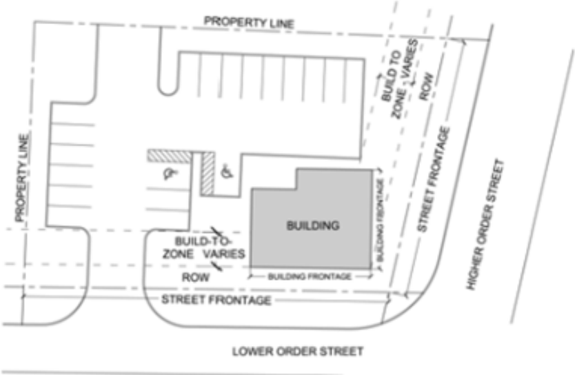
Preferred Urban layout for fueling station as shown in the City of Fayetteville’s UDC, 164.06
