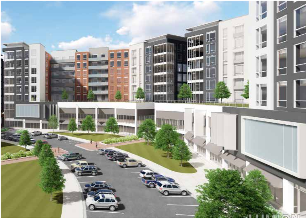
Mall redevelopment concept. In this concept, the Mall’s peripheral drive would be moved inward toward the main building and redesigned as a city street. The drive relocation opens sites for residential buildings with some street level retailing. Parking would be provided on the lower levels, served by ramps on the back side of the apartment blocks. The site affords excellent views of the forested hills and creek to the west, and has direct access to the Razorback Greenway.
