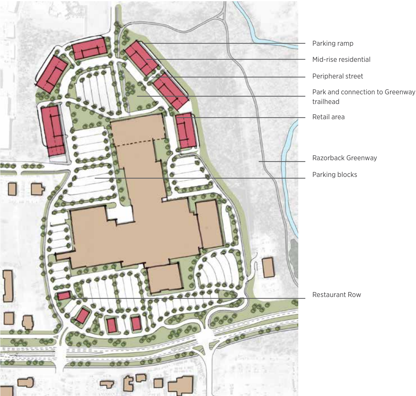
Mall redevelopment concept. In this concept, the Mall’s peripheral drive would be moved inward toward the main building and redesigned as a city street. The drive relocation opens sites for residential buildings with some street level retailing. Parking would be provided on the lower levels, served by ramps on the back side of the apartment blocks. The site affords excellent views of the forested hills and creek to the west, and has direct access to the Razorback Greenway.
