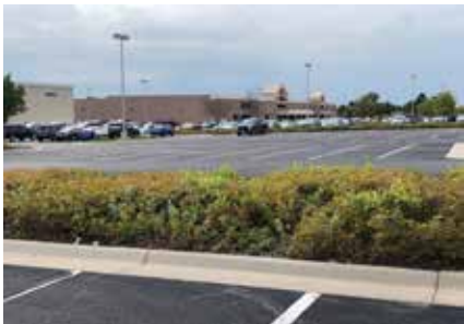
Parking bays separated by landscaped corridors. Requiring a landscaped separation between each three contiguous parking bays breaks up large expanses of parking when they occur. (Derby, KS)
