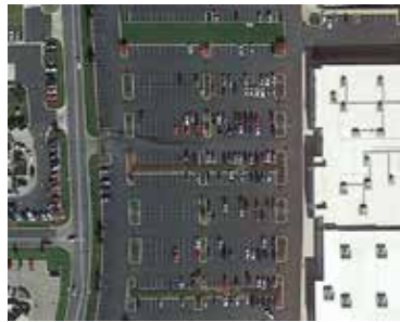
Parking bays separated by landscaped corridors. Requiring a landscaped separation between each three contiguous parking bays breaks up large expanses of parking when they occur. (Derby, KS)
