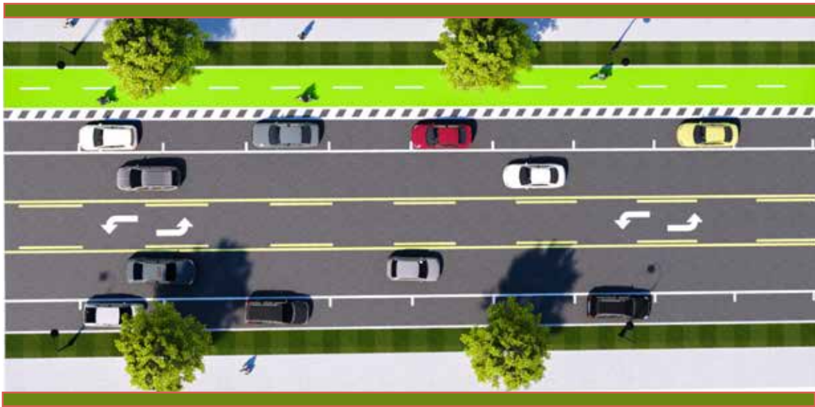
South School perspectives Right: Rendering of section with buffered directional bike (mobility) lanes. Far right: Preferred concept with two-way cycle track on west side of street and parking shoulder, with sidepath on east side. The separation between travel lanes and the bicycle facility may be accomplished by parking, a painted buffer, bollards, planters, or a raised median.
