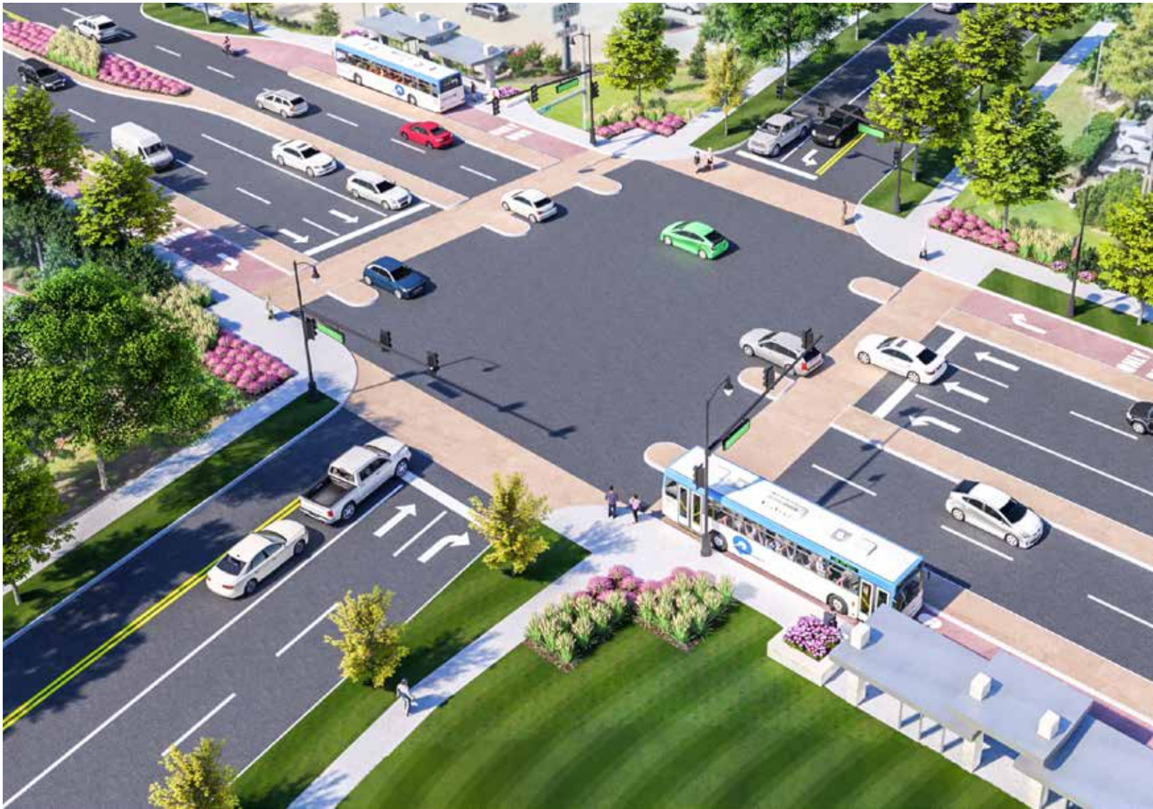
College Avenue Concept. From left: Sketch of an initial North to Township segment of the street; close-up plan of the Township intersection, illustrating bus rapid transit (BRT) and right turn only turnout lanes; and a rendering of the Township intersection. A bus turnout lane can provide room for transit to bypass a traffic queue and to control the signal at this location. This provides the BRT with a distinct time advantage over automobiles at busy intersections. Intermediate medians and a wide nose at the center median provide pedestrian refuges that break up the width of the street. A greater orientation toward transit, substantial residential development along and adjacent to the corridor, and increased use of active transportation modes could lead to a future reconsideration of the nature of College Avenue that could ultimately include enhanced transit such as light rail and more intensive development at intersections like this one. An alternative concept would place the transit stop in the outer travel lane. This avoids the increase in pedestrian crossing distance but places the BRT in the line of regular traffic, eliminating its potential time advantage at intersections.
