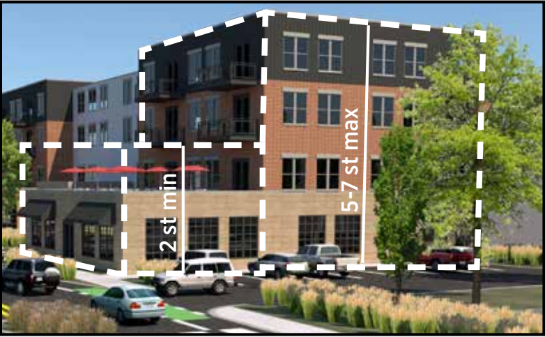
Step-back building concept at Urban Place nodes. The possible regulation permits a two (rather than three)-story minimum height at the building line, provided that the project includes a higher building, consistent with UT requirements, behind.
