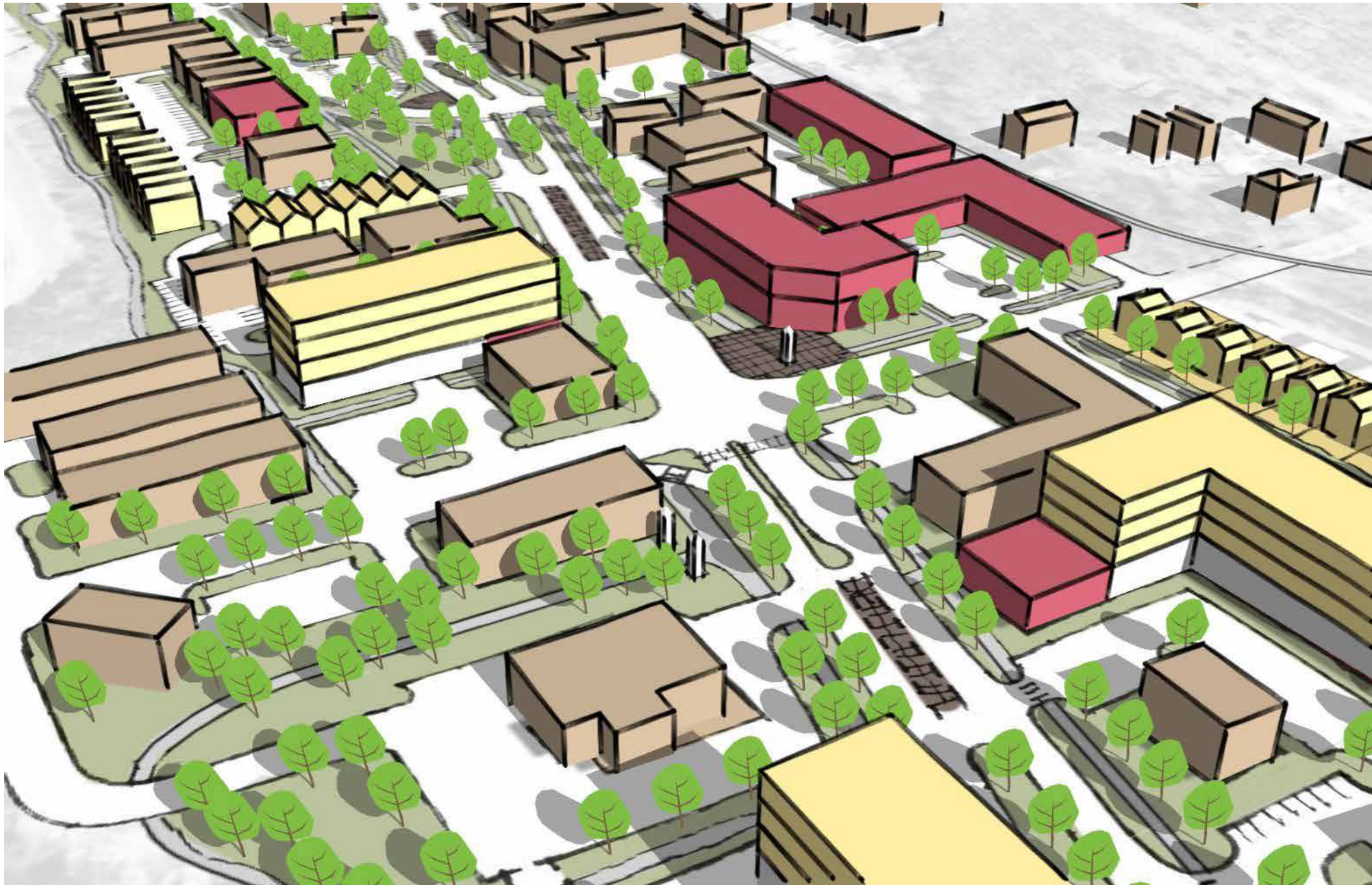
Sycamore Node. Massing diagram looks northeast, showing potential mixed use development on the northeast corner, completing a higher intensity node at the intersection. Townhouses and a green space made possible by relocating the Green Acres intersection.
