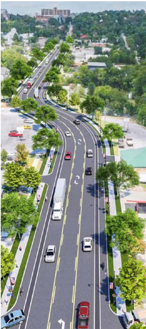
South School perspectives Right: Rendering of section with buffered directional bike (mobility) lanes. Far right: Preferred concept with two-way cycle track on west side of street and parking shoulder, with sidepath on east side. The separation between travel lanes and the bicycle facility may be accomplished by parking, a painted buffer, bollards, planters, or a raised median.
