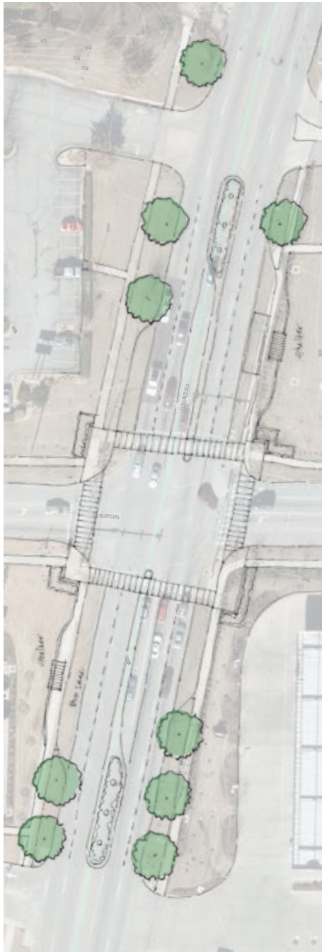
College Avenue Concept. From left: Sketch of an initial North to Township segment of the street; close-up plan of the Township intersection, illustrating bus rapid transit (BRT) and right turn only turnout lanes; and a rendering of the Township intersection. A bus turnout lane can provide room for transit to bypass a traffic queue and to control the signal at this location. This provides the BRT with a distinct time advantage over automobiles at busy intersections. Intermediate medians and a wide nose at the center median provide pedestrian refuges that break up the width of the street. A greater orientation toward transit, substantial residential development along and adjacent to the corridor, and increased use of active transportation modes could lead to a future reconsideration of the nature of College Avenue that could ultimately include enhanced transit such as light rail and more intensive development at intersections like this one. An alternative concept would place the transit stop in the outer travel lane. This avoids the increase in pedestrian crossing distance but places the BRT in the line of regular traffic, eliminating its potential time advantage at intersections.
