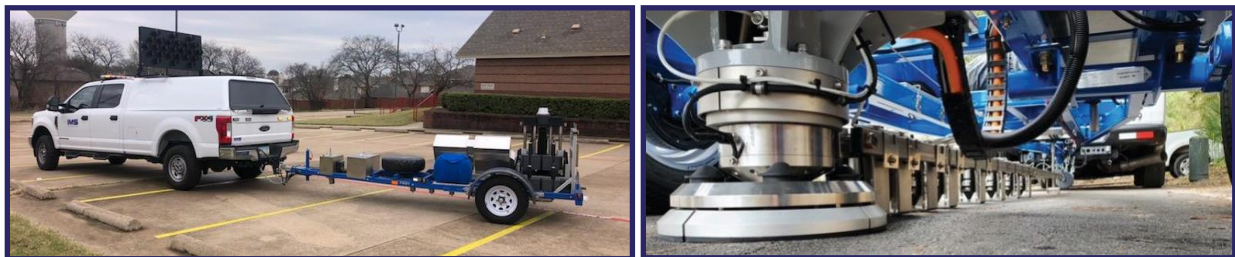
Figure 10 - Fast Falling Weight Deflectometer
